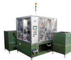
Magnetic trip unit eight-station automated resistance welding machine
