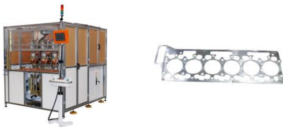
3x55KVA MFDC Automatic Welder for Car Cylinder Head Gasket
