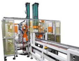
120T Clinch Machine for Wash Machine Rear Panel ZMY-120-001-16001
