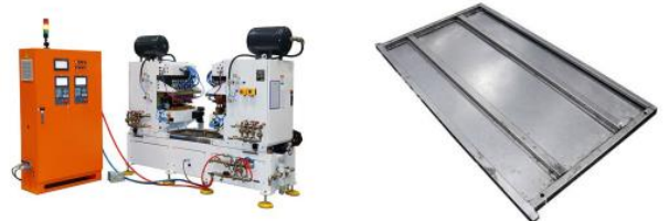
440KVA MFDC Multi Spot Welder for Supermarket Shelf Plate Strengthening Assembly DB-440-19005
