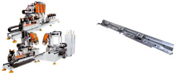
Customized Spot Welder for Car Door Threshold
