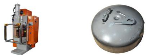
Water heater hanger welder
