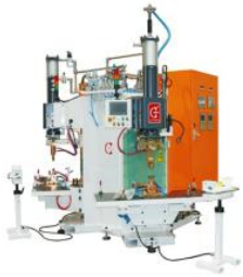
20KJ Double-Head Capacitor Discharge Projection Welder for Automobile A/B/C Pillar
