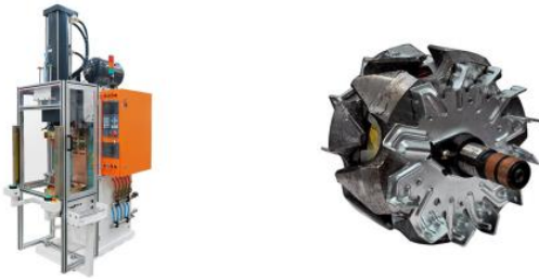
440KVA MFDC Welder for Welding Motor Fan to Rotor DB-440-20002
