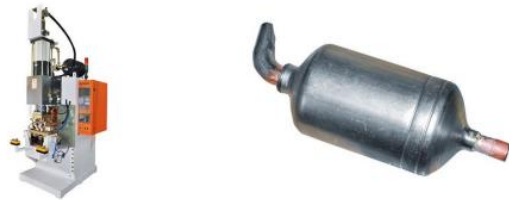
660KVA MFDC Welder for Reservoir Bend Pipe DB-660-18002
