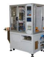
110KVA MFDC Customized Welding and Cutting Machine for Braided Copper DB-110-19003
