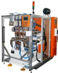
Customized MFDC Spot Welder for Automotive Door Frame Center Pillar
